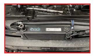
20. Install the remaining line to the cooler.
