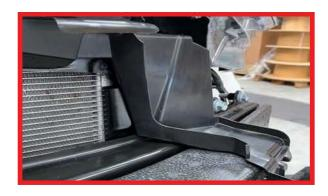
**17.** Feed the cooler lines through the space between the headlight and crash bar.
