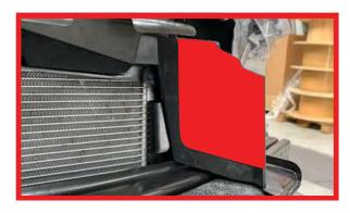
**16.** Remove the radiator shroud and trim along your cut line, then re-install to the car.
