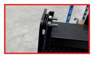
**8.** Using the supplied hardware install the cooler and bracket assembly to the two tabs in the centre of the crash bar. Ensure that the washers are in the correct orientation (bolt - spring washer - flat washer).
