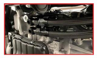
**22.** Check the routing of the hoses for clearance and potential chaffing areas. Install the two supplied hose separators where required. \*use the photos below as a guideline.
