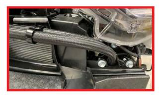
**18.** Using new engine oil, fill the cooler to just below the threads (approx 0.4L).
