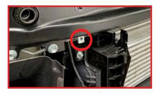
**6.** Fit the horn to the new location using the supplied bolt and washer. Re-connect the horn wiring harness.
