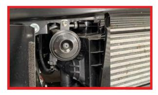
**7.** Install the cooler to the mounting bracket using the supplied bolts, O-rings and nuts.
