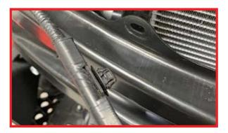
**5.** Route the horn wiring harness below the headlight and down behind the crash bar, then install the supplied chimney nut to the highlighted tab.
